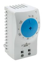
The mechanical NO thermostat closes when the temperature rises and is used to control filter fans, heat exchangers, cooling devices or to switch signal transmitters when the temperature is exceeded. The use of push-in terminals prevents the supply lines from coming loose.
